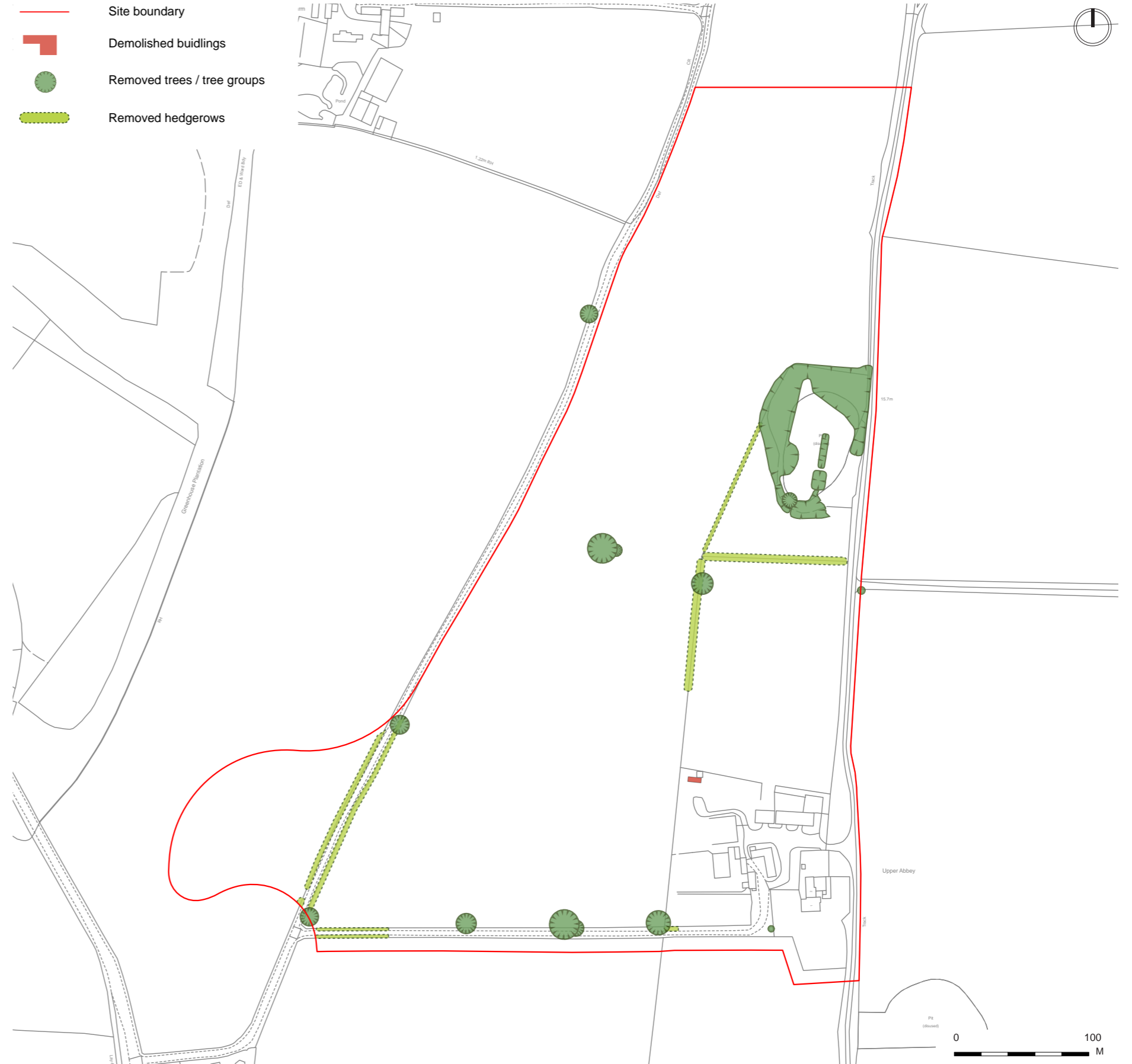
Figure A.57: Clearance and Demolition Plan
