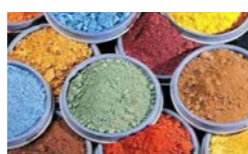
Concrete colour can be influenced by pigmentation addition
